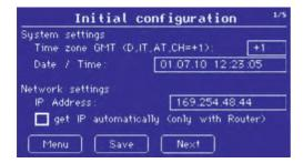
The time is important. It is factory-set but can be lost after a long time in storage. In this case, the value is random and must be corrected.
