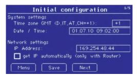
Be sure to check the date and time. The STL800 contains a backup capacitor, which backs up the factory-set time even after a long time. Nevertheless, you should adjust the date and time if necessary. You can also set the IP address of the STL800 to speed up access to the STL800 from your PC. Alternatively, you can configure the address later. See the section "Connecting to a PC/network." If the STL800 is connected to an Internet router, the network address can also be configured automatically.
