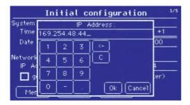
The virtual keyboard opens on the display as needed, and you can enter information similar to using a real keyboard. A small numerical keypad or a full alphanumeric keyboard is displayed depending on the type of text to enter.
