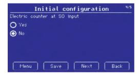
If an electricity meter is connected to the SO input, this dialog box is where you enable that meter. This information is important since the STL800 manages the electricity meter as a virtual inverter. An electricity meter "inverter" will always be number 1; all additional "real" inverters follow.
