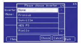
The RS485/422-B interface is defined in the third dialog box, where you also define settings for Fronius inverters.
