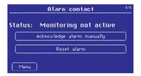
The STL800 constantly monitors its internal alarm contact. As soon as the contact is broken, an alarm is triggered. You can configure what happens in this event in the "Config./ Advanced/Alarm contact" dialog box (email/relay notification).
