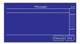
The STL800 generates messages when errors and faults occur or only about the current daily yield depending on the configuration. Every message can se be sent as an email. All messages are also cached and can be opened on the display. You can open the 50 most recent messages. Opening the list of messages acknowledges a connected relay triggered by system monitoring.
