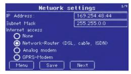
This dialog box lets you configure the IP address and subnet mask of the STL800. The factory-set address is 192.168.178.49 and must be changed to enable access from a PC. For a detailed description of what needs to be done, see page 61.
