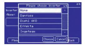
In the second dialog box, you can specify the manufacturer of the inverter connected to the RS485-A interface. Note that the SMA SensorBox is treated like an inverter and is therefore listed under inverter type SMA.
