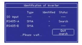
Every interface is shown with the pre-defined inverter type, and everything is searched in sequence. This process can take a relatively long time. For example, if you have Sputnik/SolarMax inverters, an address range of 253 addresses is searched.
