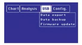
You can back up data on your USB stick or to the data logger at any time. All data (daily curves up to 60 days), i.e. configuration and measurement data, is always saved.
