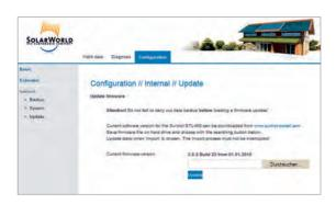
This item lets you update the STL200/400 software, which lets you integrate new functions into the system at any time or eliminate errors.
