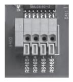
Connect the individual inverters together via the RS485 terminal blocks using a shielded, 2-pin data cable as described in the Sunways manual. Each inverter has two RS485 ports to enable the inverters to be connected in a series.
